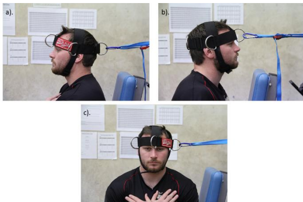
Figure 1: Experimental set up for testing players isometric MVC in a) flexion, b) extension, and c) right lateral flexion.
